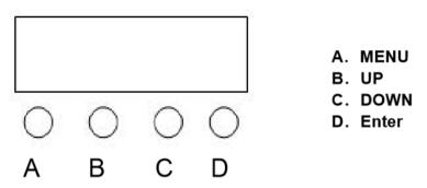
**Operation description:** Press "A" will cycle out seven different functional effect, LED Top row in represent the current function (Reference function table). LED Top row on behalf of the function in the address code, or speed and other parameters. Press  $\bf B$  or  $\bf C$  key can modify the parameter value. Press  $\bf D$  to confirm.
